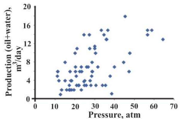
**Figure 10.** The chart of dependence between daily average volume of extracted fluid (oil+water) and formation pressure on Neft Dashlary field
