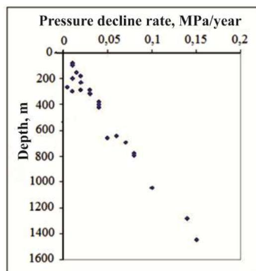
Figure 3. Rate of fall of formation pressures vs. depth in Balakhany-Sabunchu-Ramana field
