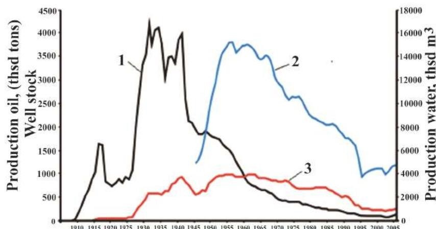
Figure 8. Surakhany field: dynamics of main operating parameters: 1 – oil; 2 – water; 3 – number of wells
