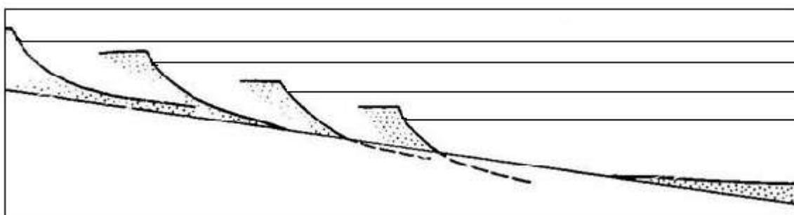
**Figure 1.** Erosion of the underwater shoreface during rise of the sea level (according to Zenkovich, 1962)
