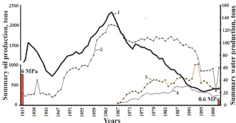
**Figure 5.** Development diagrams of the Horizon VI (Balakhany suite) of Balakhany-Sabunchu-Ramana field: 1 – oil production; 2 – water production; 3 – volume of injected water; 4 - number of injection wells
