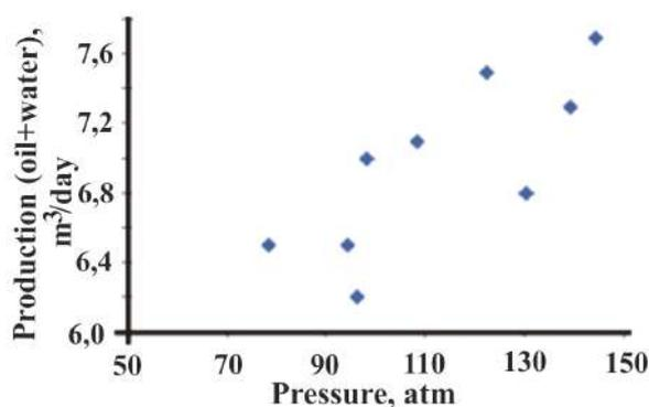
**Figure 9.** Dependence between average daily extracted volume of fluid (oil + water) and formation pressure on Buzovna-Mashtaga field
