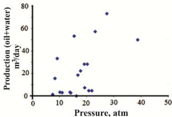
**Figure 4.** The graph of the relationship between average daily volume of the fluid (oil + water) extracted from the reservoir and formation pressure in Balakhany-Sabunchu-Ramana field
