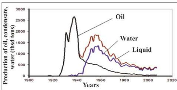
Figure 6. Main operating parameters of the lower parts of PGS, Balakhany-Sabunchu-Ramana field
