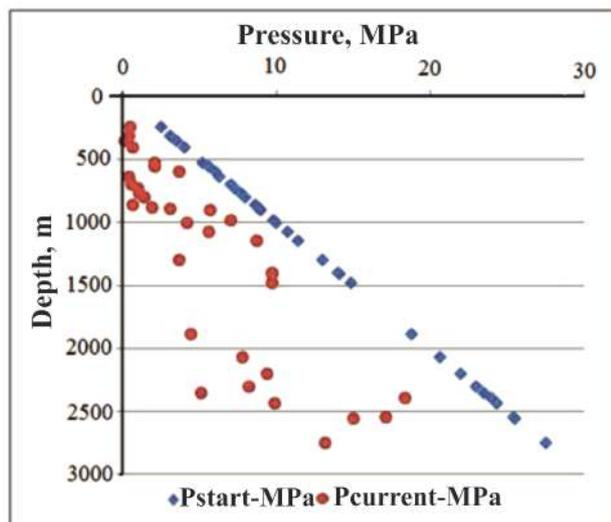
Figure 7. Initial and current formation pressures in Surakhany field vs. depth
