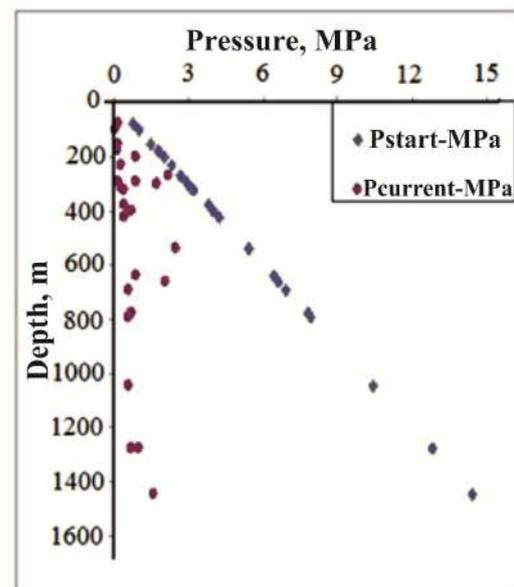
Figure 2. Initial and current formation pressures in Balakhany-Sabunchu-Ramany field vs. depth
